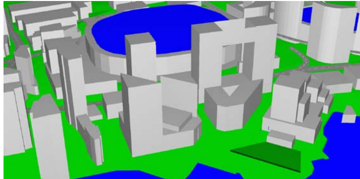
Figure 2: 3D view of Cadna/A noise model showing some of the modelled roads, BC Place, existing buildings, the proposed audience area in dark green and proposed building layout.
